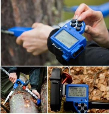
The DPII is suited for log scaling. with jaws designed for easy placing in between and under logs. The Smart Scale<sup>TM</sup> and the data terminal can be used as standalone instruments – use the scale as a manual caliper, and send wireless diameter data to the terminal. If you work with the Digitech Professional Caliper and wish to update your equipment your software can be adapted for the DPII.
