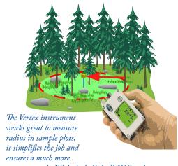
accurate result. With the built in BAF function you are able to be at the tree and determine its minimum diameter to be included into the point. The BAF function allows you to conduct accurate point samples on tracks with thick underbrush where traditional prisms fail.
