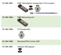
**The Transponder T3** is used together with the Vertex, the Vertex Laser and the DME. It is water resistant, rugged and has a simple construction in a bright, visible color. Works with one AA battery. Pin transponder on the tree stem or use the adapter on the custom monopod to measure in circular plots. Diameter: 70mm. Weight: 85 g. 1 x 1.5V AA alkaline battery, consumption max. 9mW.
